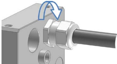
Before connecting clean the flat mating surface to avoid inclusion of contamination. Connect and disconnect in according to the instruction of use for multicoupling. Test the correct functioning of the electrical connector.
