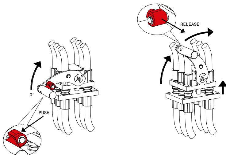
Continue to rotate till the safety lock automatically engage itself in the 12 o 'clock position. Pull out mobile half from fixed half pins.(Pay attention during the pulling phase not to make the mobile half fall down causing injure).
