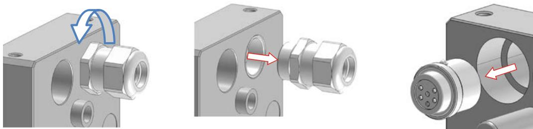
Unscrew the plastic nut from the cable retainer, then insert the cable in the plastic cable retainer, so strip the cable for a length of 30 mm and the single wires for 10 mm.
