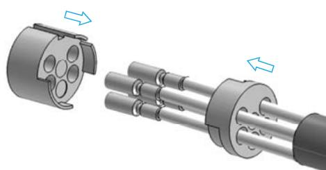
Insert the metal body of the electrical connector at the back of the multicoupling. Insert the cable with all the group assembled on.
