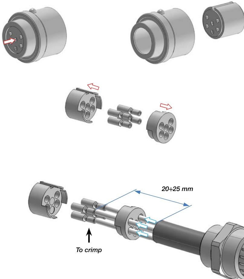
Assemble the cartridge with all the pins & wiring crimped.
