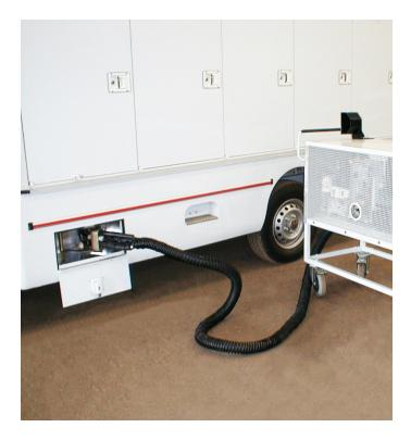
Thanks to the multicoupling these **three** main lines are connected and disconnected simultaneously by a single and quick movement.
