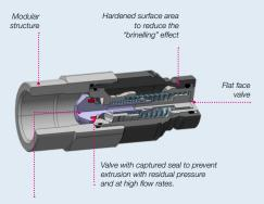
Internal check valve without pressure eliminator to close the circuit in case of accidental releasing of the pressure in the female side.
